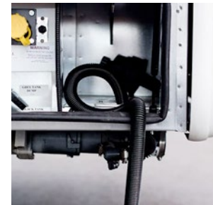
Macerator Sewage Discharge c/w Manual Disconnect
