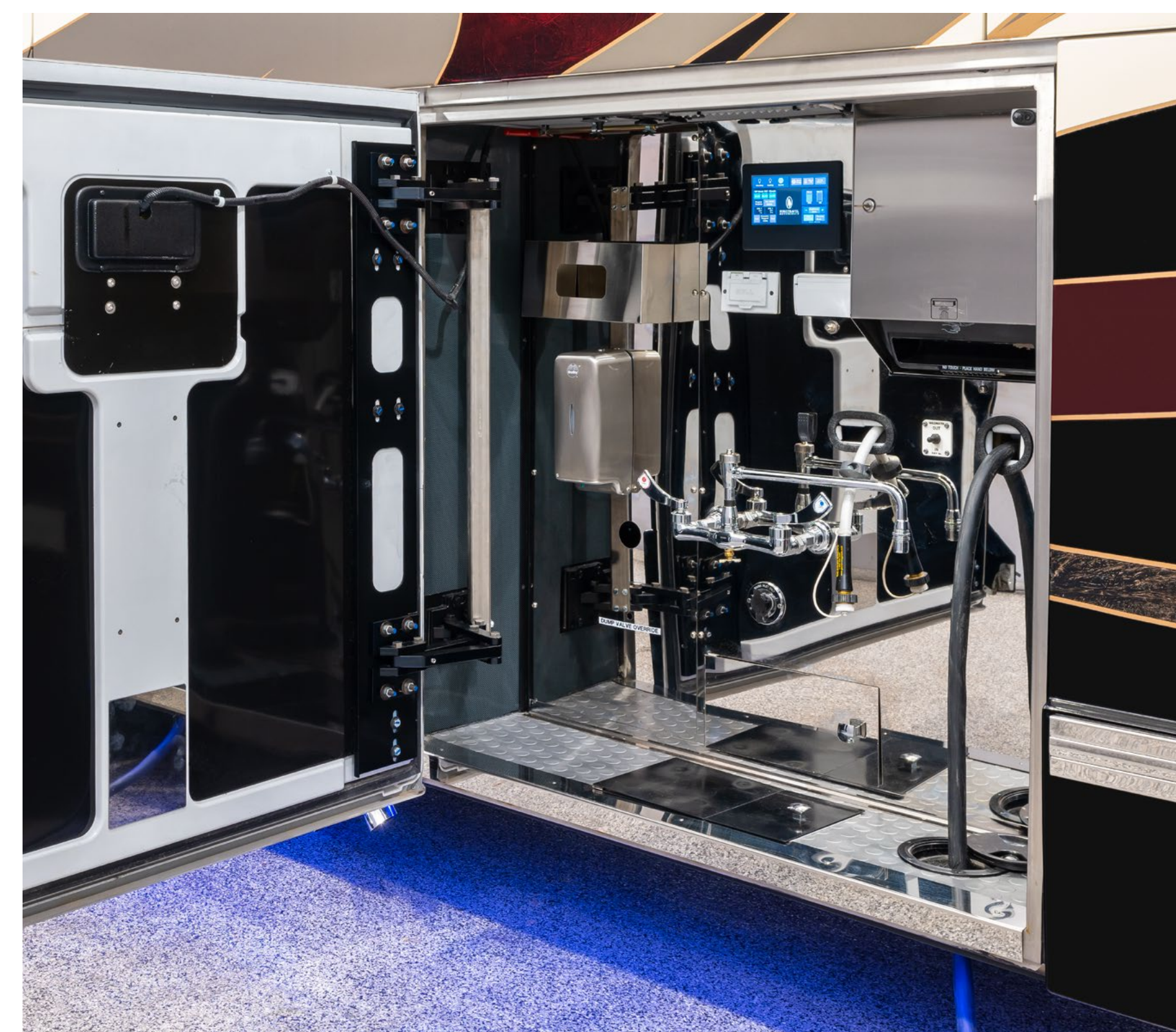
Fully equipped external wet bay
