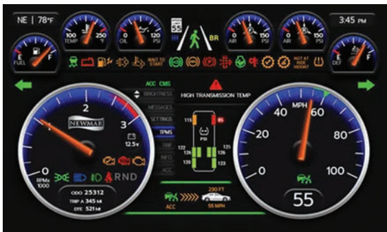
Spartan’s Digital Dash allows owners to quickly and easily check the status of their tires (on models equipped with TPMS), oil pressure, coolant, etc.
