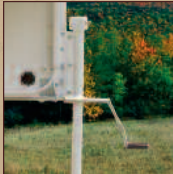
Four 2,000 lbs. manual ball screw jacks allow for easy leveling
