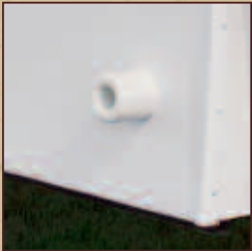
Front rubber bumpers protect the front of the truck bed.
