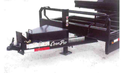
Top: 17.5" H-rated tires Bottom: Standard tool box and adjustable coupler
