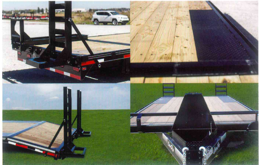
Top left: Standard stand up ramps Top right: Plated wheel well for lower profile Bottom left: Optional full/split gates Bottom right: Optional front tool box
