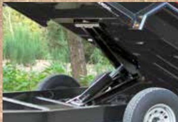
Scissors Hoist Standard on 12' & 14' (cylinder on 10')
