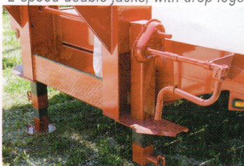
2-speed double jacks, with drop legs
